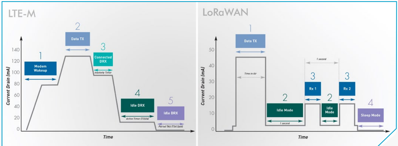
Figure 12: Typical power consumption of a LTE-M based module and a LoRaWAN based module
